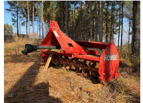
A 3-point hitch rototiller can be a great tool for food plot planting and fire break maintenance. Photo credit: Stephen Pohlman, Clemson Extension.
