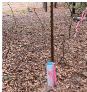
Large PVC pipe is driven in the ground over a corner iron. Photo credit: Janet Steele, Clemson Extension.
