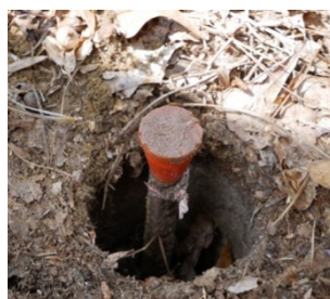
Rebar is a typical marker for property corners. It often has a plastic cap on top stamped for the surveyor who set the iron. The type of marker will be noted in the deed description or in the plat legend. Photo credit: Janet Steele, Clemson Extension.
