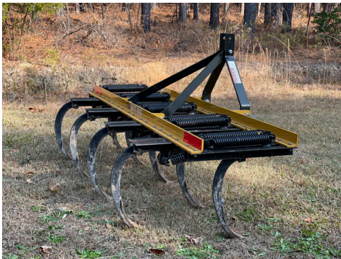
This shank-style plow is referred to by many names such as an All-Purpose plow, spring-shank field cultivator, ripper plow, chisel plow, and spring-tooth scarifier. Photo credit: Stephen Pohlman, Clemson Extension.
