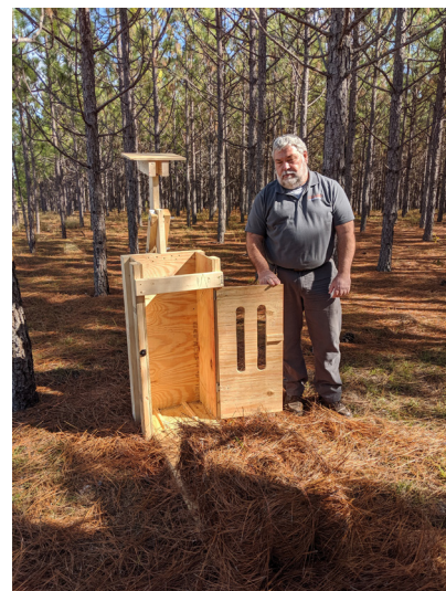
Pine straw box baler. Photo Credit: Ryan Bean, Clemson Extension
