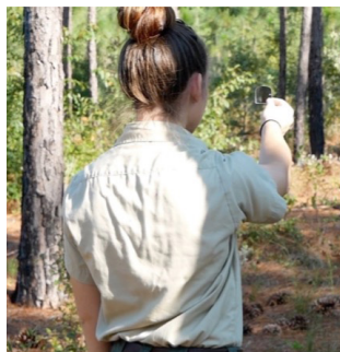
Figure 3. A wedge prism is used to determine basal area. Photo credit: Janet Steele, Clemson Extension.
