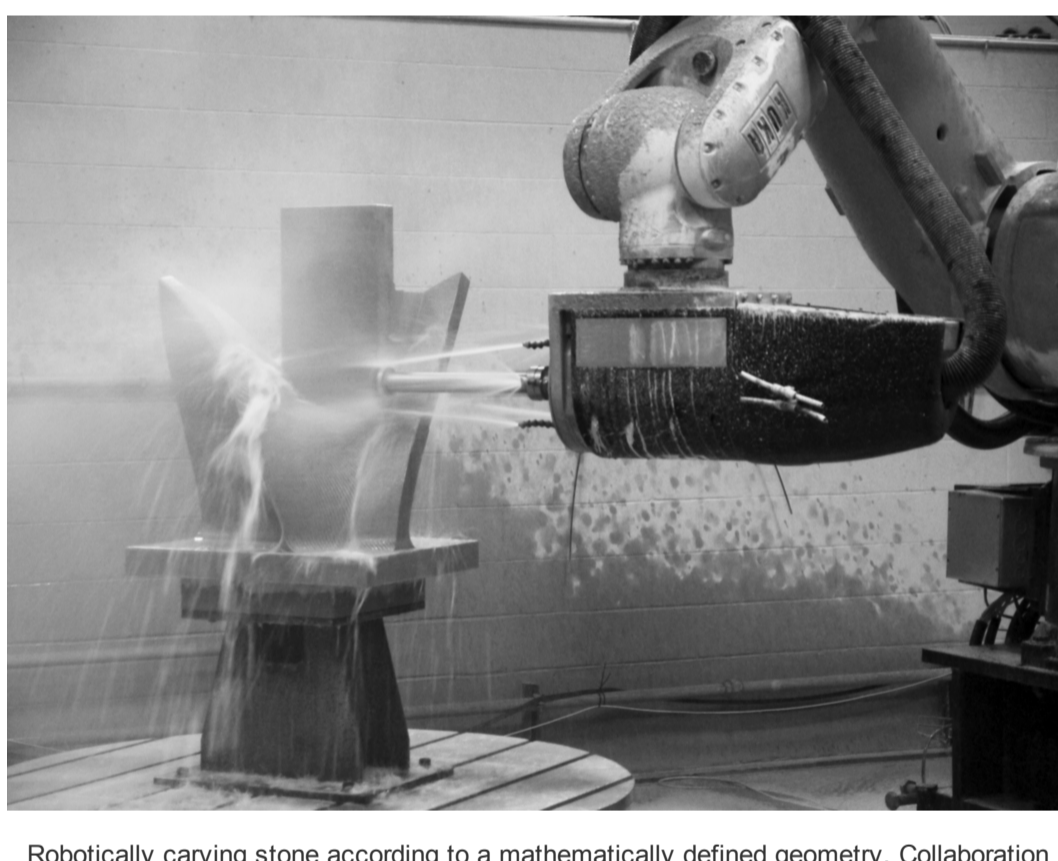
Robotically carving stone according to a mathematically defined geometry. Collaboration between Professor Choma and Quarra Stone Company.
