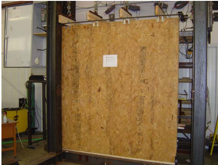
Photograph shows the test set-up to investigate the performance of roof-to-wall connections under combined cyclic uplift and in-plane shear loads. A computer controlled screw drive actuator simultaneously applies the uplift and shear loads to the roof framing.
