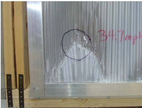
Photograph shows impact damage to a hurricane shutter from a 9-lb 2x4 missile traveling approximately 34 mph.
