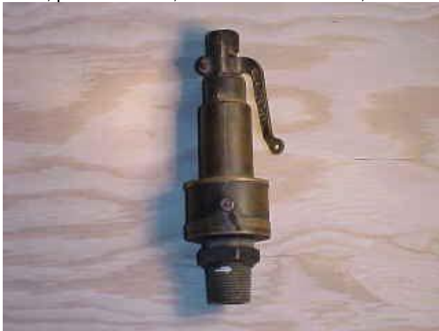
Valve, pressure relief, 3/4-inch male threaded, brass
