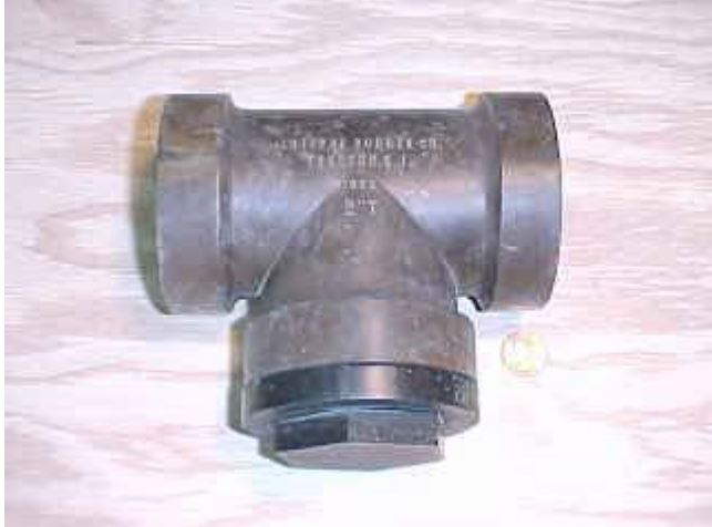
Valve, ball check, 2-inch, threaded, hard rubber
