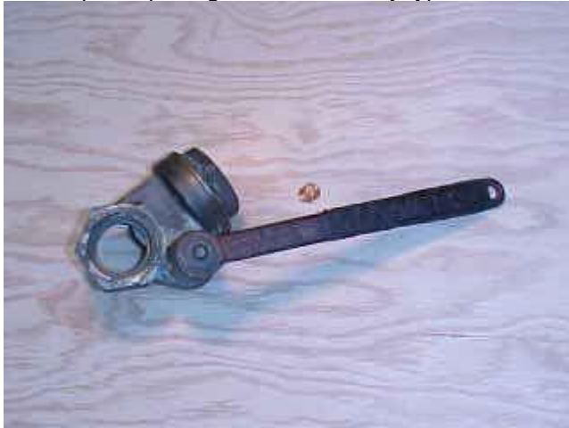
Valve, globe, lock type, ½-inch, union slip-welded ends, brass
