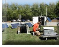
The **Lee** research group deployed a distributed sensor system (DTS) along Town Creek near the Sangamo Weston Superfund site. Over a kilometer of fiber optic cable will be placed in the stream and used to measure temperature changes. The system will identify groundwater flux and possibly fractures within the stream bed. **David Hahn** (MS, Hydrogeology) tested the system before taking it on site along Town Creek.
