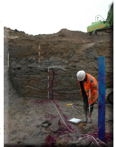
Vertical hydraulic fracture filled with rhodamine dye in glacial till. From former graduate student Chapman Ross , now at Geosyntec
