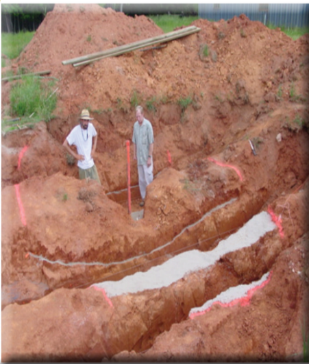
Hydraulic fracture created in Piedmont residual soils by former graduate student Jim Richardson
