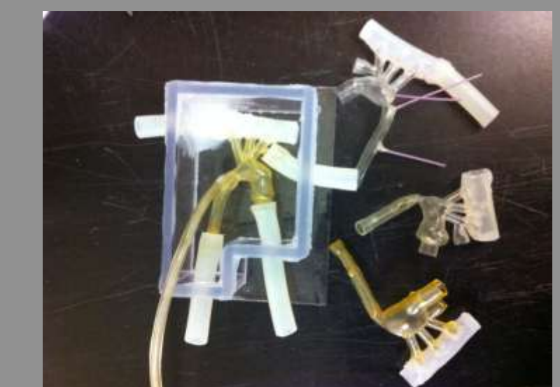
FIGURE 8. Patient specific aorta test section with different geometry
