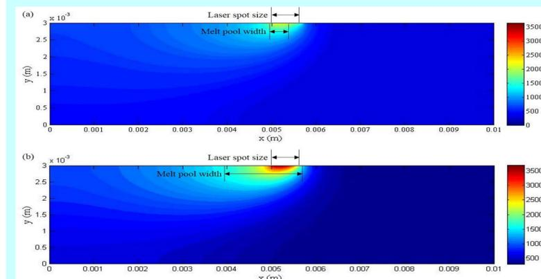
Laser moving at 10 mm/s on Inconel 718, with laser power: (a) 75 W, and (b) 150W
