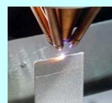
LENS process with powders injecting into the melt pool
