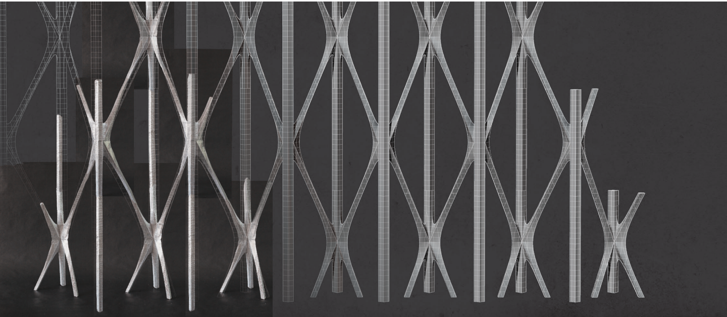
1 Lattice system cast from 3D-printed ceramic molds (Authors 2018).
