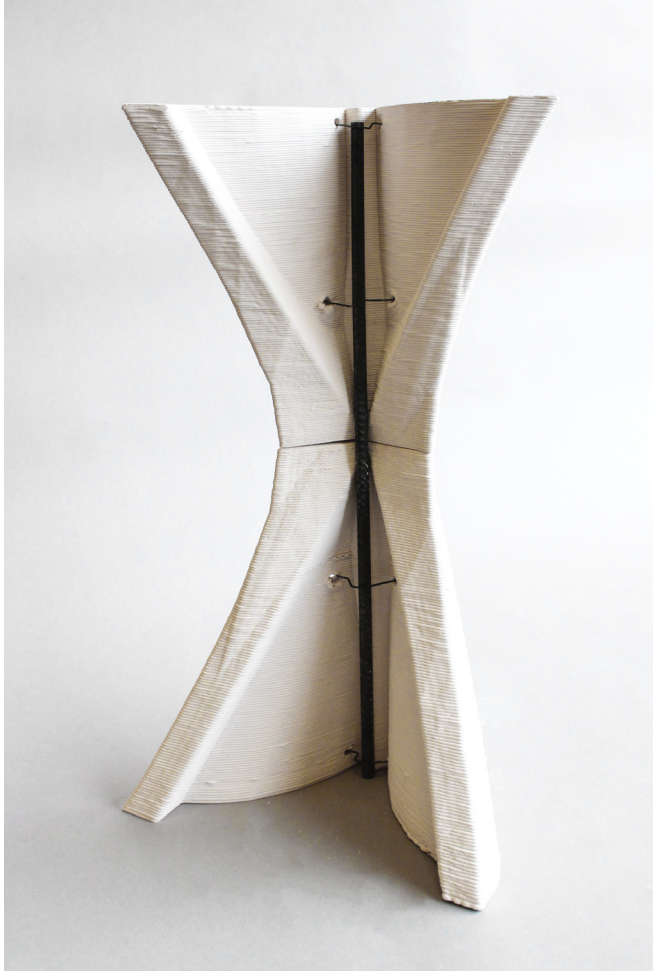
2 Two piece 3D-printed ceramic mold (Authors 2018).
