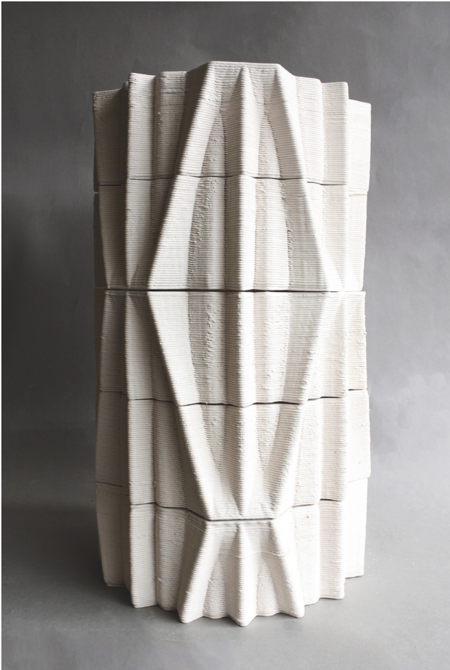
13 Lattice column multi-piece stacked ceramic molds (Authors 2018).
