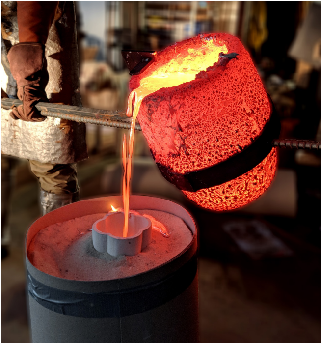
9 Pouring aluminum into 3D-printed ceramic mold (Authors 2018).
