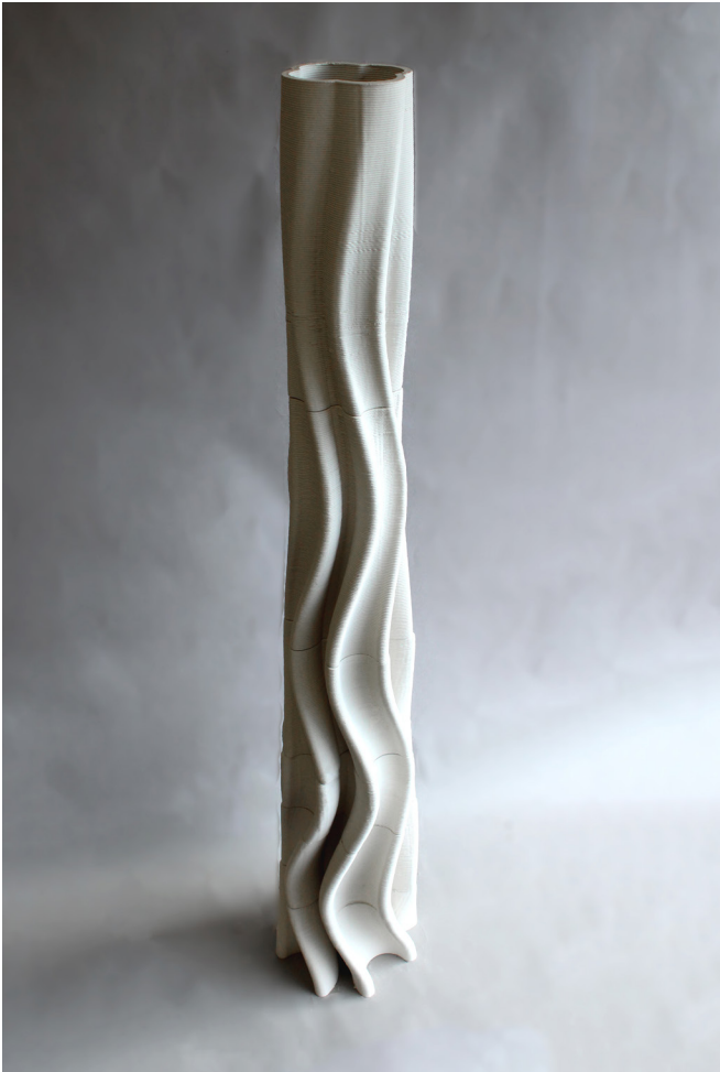
7 3D-printed ceramic mold for Column (Authors 2018).
