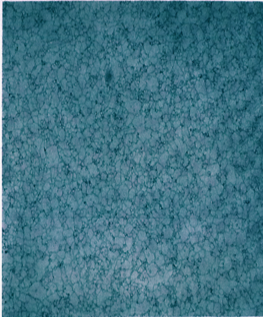
Figure 7. Microstructure of MICRO-GRAIN™ ZIMALOY®. Note: Grain size is ASTM 12
