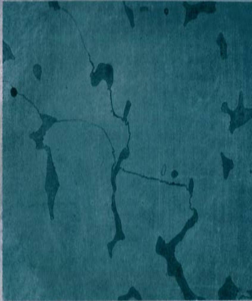
Figure 6. Microstructure of investment cast Co-Cr-Mo alloy. Note: Portions of three grains are observed.
