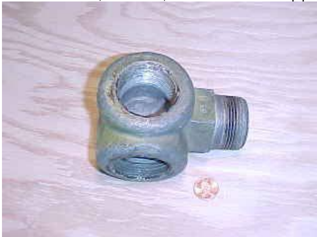
Elbow 1-1/4-inch, aluminum, with 1-1/4-inch male pipe side outlet.
