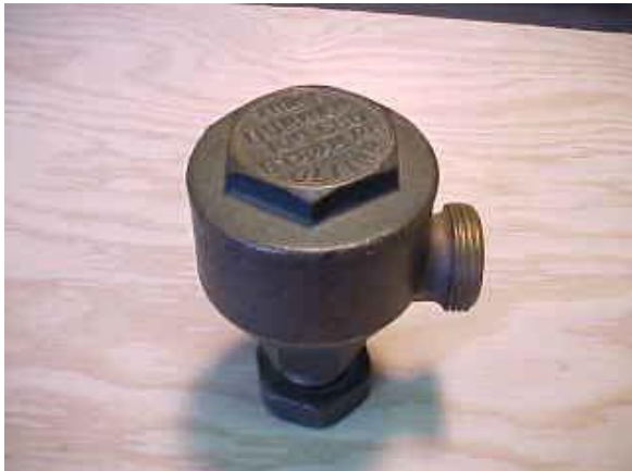
Thermowell, 3/4-inch, for Weston thermometer, SS
