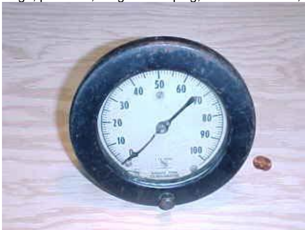
Gage, pressure, range 0-100 psig, 1 lb. increments, recessed panel mounting, 1/4-inch threaded
