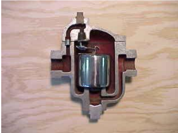
Steam trap, bellows type, 3/4-inch, brass
