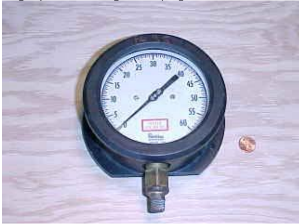
Gage, pressure range 0-60 psig, 1 lb. increments, flush panel mounting, 1/4-inch threaded
