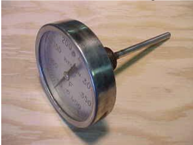
Thermometer, industrial armored type, with thermowell, range 40-110 degrees F
