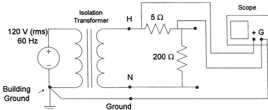
Figure B.6: Illustration of valid circuit measurement due to the use of isolation transformer.
