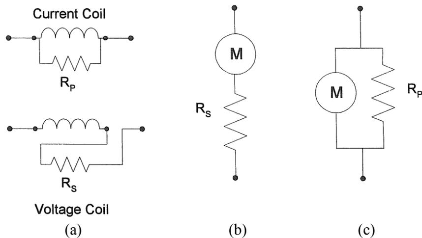
Figure B.10: (a) Equivalent circuit for analog wattmeter. (b) Equivalent circuit for analog voltmeter. (c) Equivalent circuit for analog ammeter.
