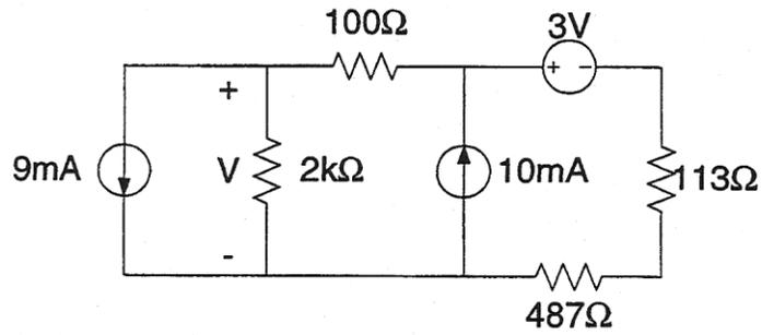
3. For the following circuit below, find the Thévenin equivalent circuit as seen at A-B.
