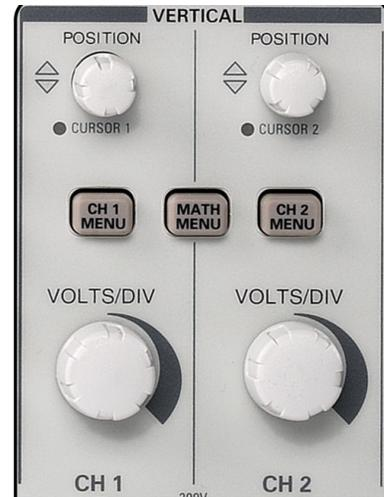
Figure E.3: Vertical Control Section
