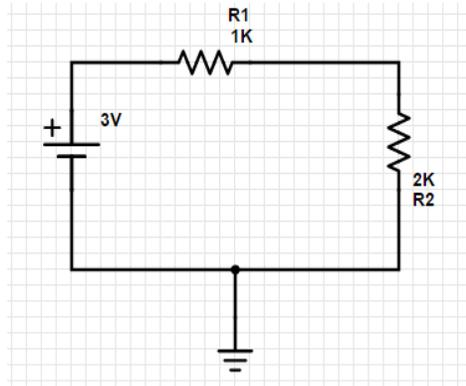
Figure F.5: Schematic of a simple circuit
