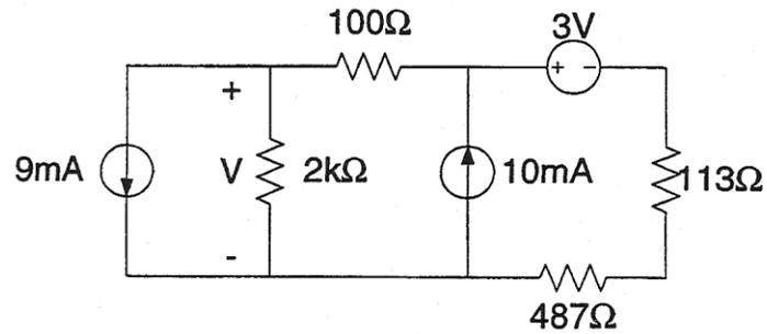
3. For the following circuit below, find the Thévenin equivalent circuit as seen at A-B.
