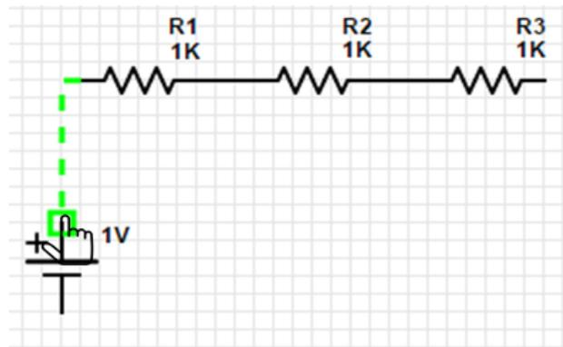
Figure F.4: Drawing wires in PartSim
