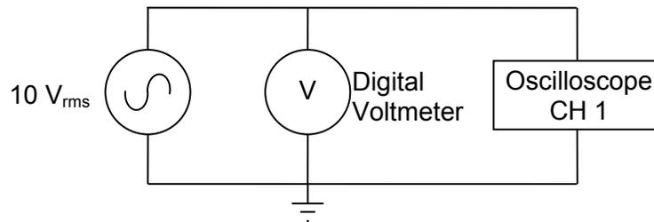
With the autotransformer turned to zero, turn on its power switch. Gradually increase the output voltage until the digital AC voltmeter indicates the output is 10 V. Record the exact value. Observe the waveform on the oscilloscope and compare the DMM reading with the peak voltage (that is, ½ the peak-to-peak voltage) measured with the oscilloscope. For a sine wave, the peak voltage,  $V_p$ , as seen on the oscilloscope, should be  $\sqrt{2}$  times the voltmeter reading,  $V_{rms}$ :
