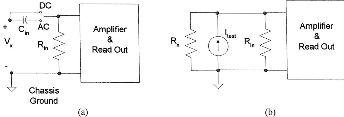
Figure B.11 (a) Equivalent circuit for voltage and current measurement with the DMM.
