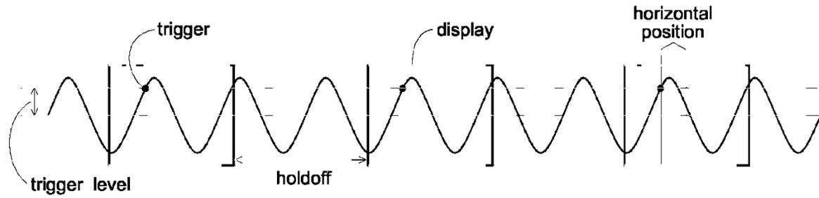
**Figure E.1:** An oscilloscope displays one wave section after another, making an apparently steady display. Determining when to start a new wave section is called triggering, and the trigger point is set by specifying the signal's level and slope (rising or falling). The trigger point is placed in the center of the display, but it can be moved using the horizontal POSITION knob. The holdoff is an adjustable dead time following a triggered wave section.
