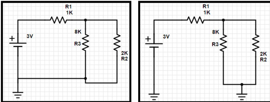
Figure F.7: The figure on the right is preferred to the one on the left.
