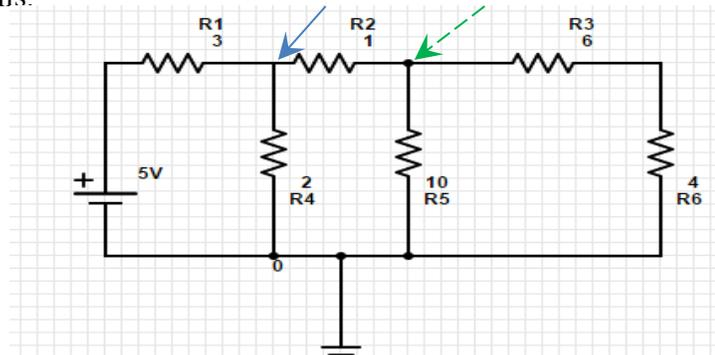
Figure F.8: The solid arrow points to a ‘not properly connected’ node
