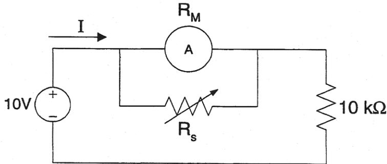
**Theoretical Question:** (DO NOT TEST THIS EXPERIMENTALLY!) If  $R_S$  were removed and if the  $10 \text{ k}\Omega$  resistor were replaced by zero ohms ( $0 \Omega$ ), what would be the current  $I$ ?
