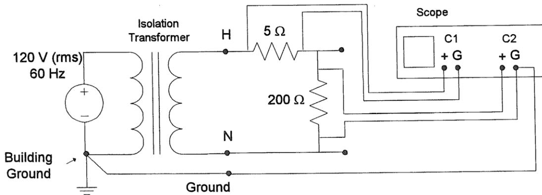
Figure B.7 Illustration of invalid circuit measurements when using isolation transformer.
