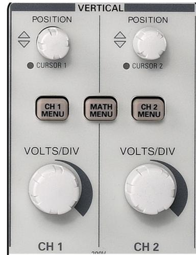
Figure E.3: Vertical Control Section
