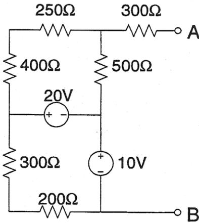
3. Use the principle of superposition to calculate the voltages across all of the resistors in the circuit below.
