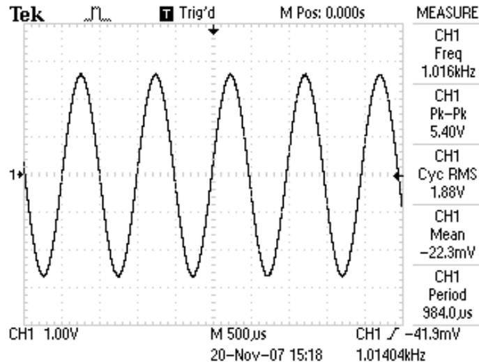
Figure E.8: Typical display. Note: MEASURE display; CH 1 V/div; horizontal time per div; trigger information; trigger point “Trig’d”.
