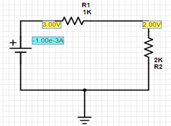
Figure F.6: We can see 2.00V and 3.00V at two nodes. The current is 1mA. The negative sign indicates that the current is coming out of the voltage source (it is delivering power).
