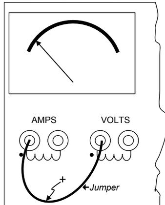
Figure B.14: Jumper on wattmeter “+” connection
