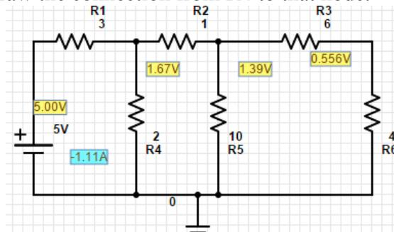
Figure F.10: R4 is properly connected.
