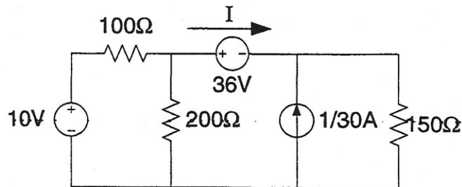
2. Apply nodal analysis to the following circuit to determine the voltage  $V$ .
