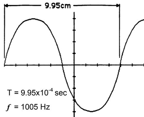
100  $\mu\text{sec/cm}$ . The period is  $T = (9.95) \cdot (100 \times 10^{-6}) \text{sec}$ . The measured frequency is  $f = 1/T = 1005 \text{ Hz}$ .
