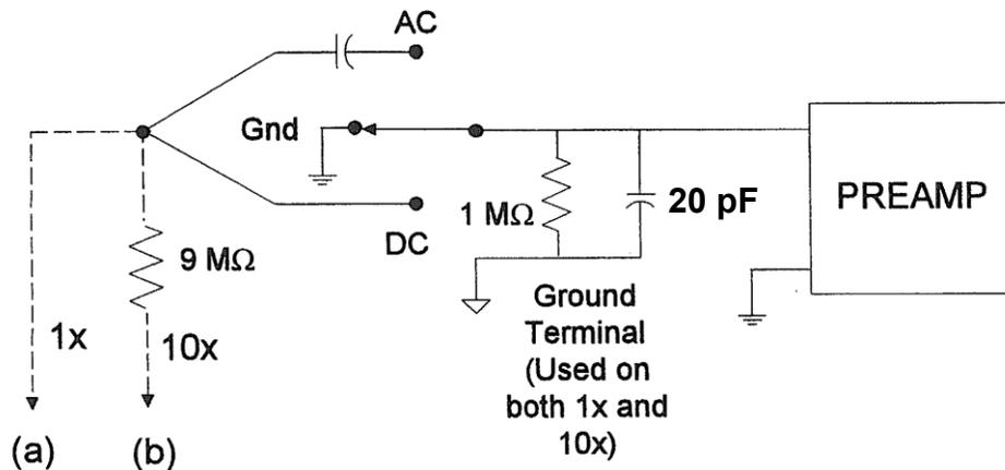
Figure B.12: (a) Equivalent circuit for oscilloscope input with 1X probe (direct input).
