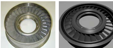
Actual (left) and modeled (right) turbine blades. Maintenance students use models in virtual reality to practice blade inspection.
