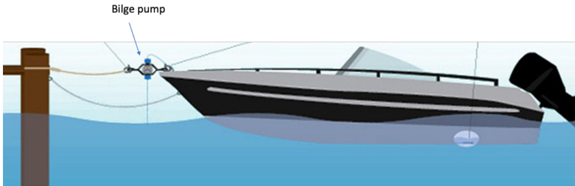
Figure 2. Bilge pump in line with mooring lines connection boat to dock.
