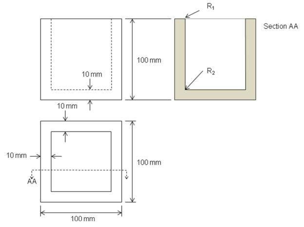
You will start with a block of 6061-T6 aluminum that is already milled to the dimensions of 100 mm X 100 mm X 100 mm and use a diamond coated high speed steel ball mill cutter with a 10 mm diameter. The bottom of the pocket should have a peak to valley surface finish ( $R_t$ ) of no more than 1  $\mu$ m. You should minimize the machining time for this operation. Please provide the following information for the pocket milling operation:
