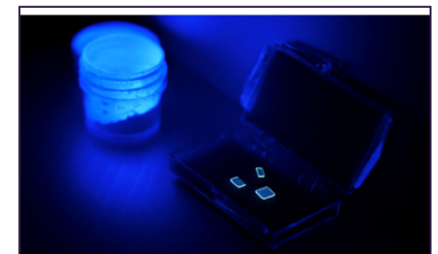
Scintillators, Dosimeters Ionizing radiation interaction with matter Photoluminescence, Lifetime, Radioluminescence, Thermoluminescence, OSL
