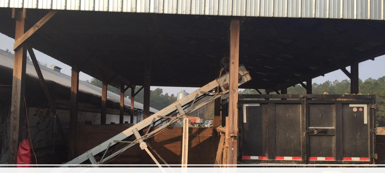
Raw material loaded into dump trailer
