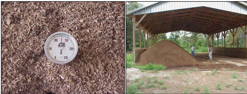
Figure 3. Windrow temperature measurements using a long-stem thermometer.
