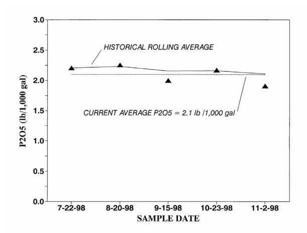
Figure 3.2. Variation in total phosphorous in the top layer of a swine manure storage pond (same samples as Figure 3.1).
