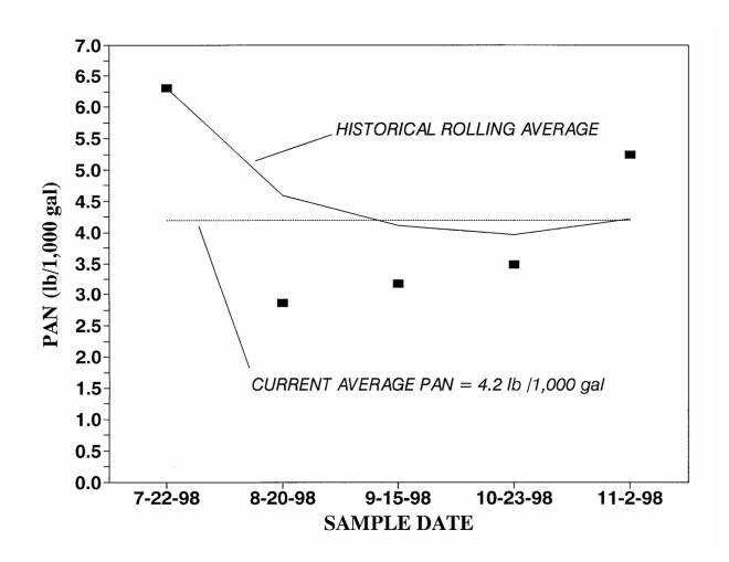
Figure 3.1. Variation in the plant available nitrogen in the top layer (1 ft) of a storage pond used to store liquid swine manure.
