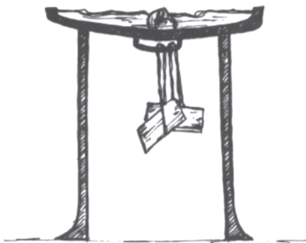
Garbage can lid, weighted with bricks on a section of drain tile.
