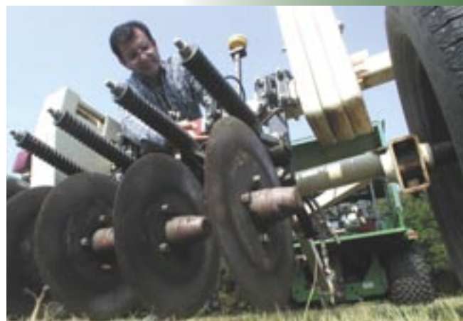
Ahmad Khalilian measures electrical conductivity in the soil to map the use of fertilizer, pesticides, irrigation and tilling.
