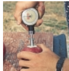
Use a penetrometer to determine apple maturity. The device works on the principle that as the flesh ripens, the fruit will become softer.
