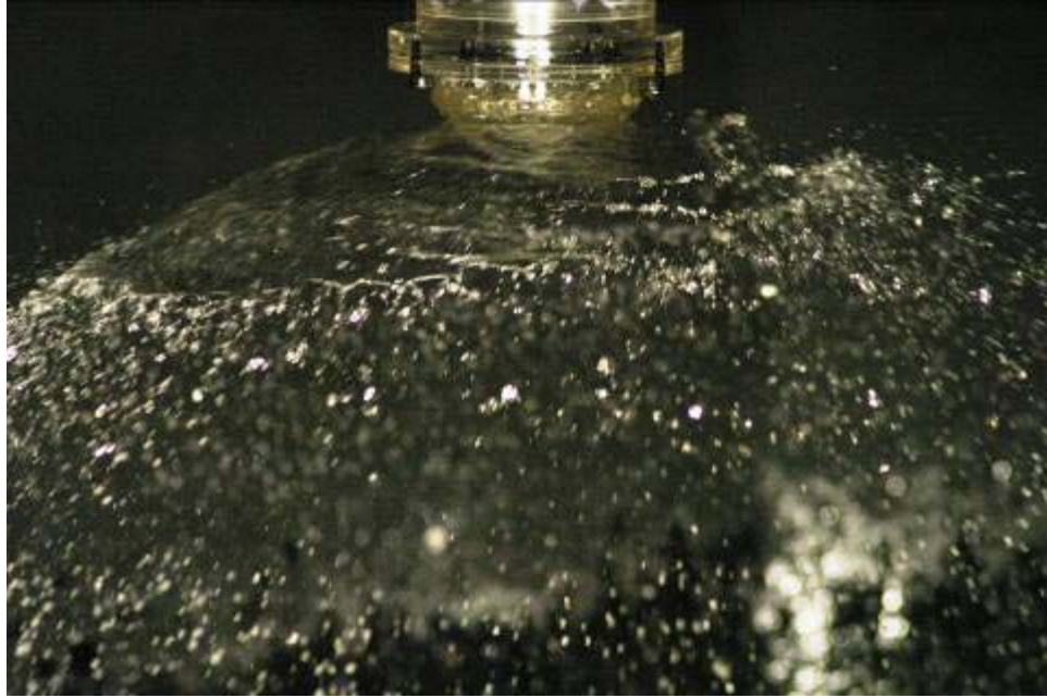
Figure 2 – Sample spray at 50 psig
