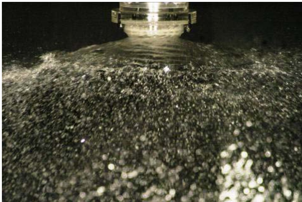
Figure 3 – Sample spray at 100 psig
