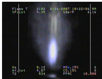
Figure 8: Photograph of the hydrogen doped pilot near blow out conditions at a flame temperature of 2280°F.
