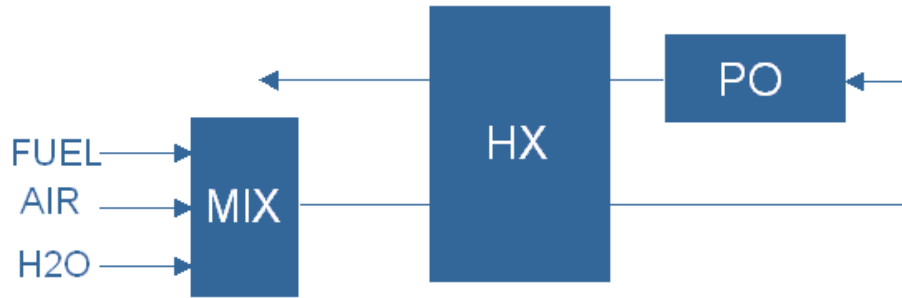
Figure 2 Schematic of auto-thermal reformation system modeled.
