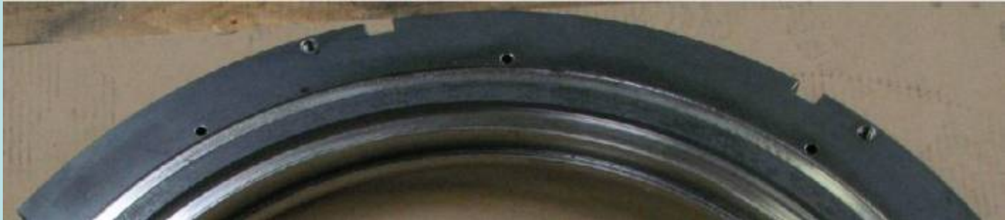
Discoloration of Semi-finished nozzle support ring
