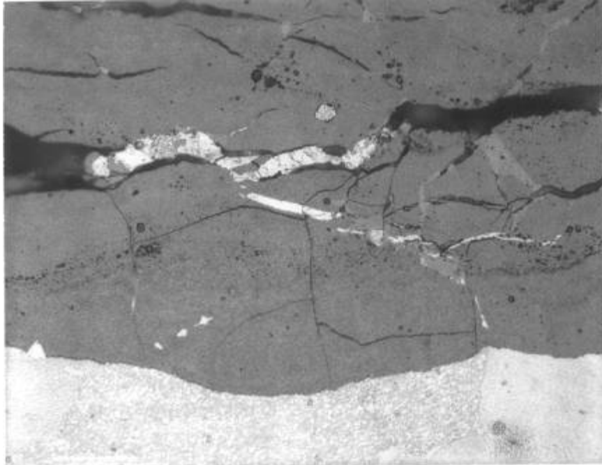
Figure 1: The microstructure of Type II hot corrosion attack
