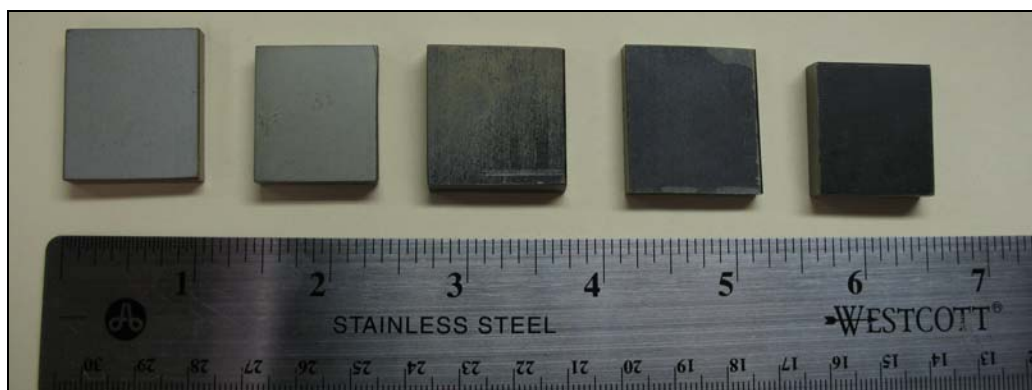
Figure 2: Polished, lightly polished and unpolished samples of a part with black discoloration
