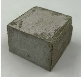
Test pieces for iron reaction with iron embedded in the mortar
