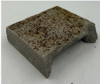
Final product is rust sprayed onto concrete to give rustic look
