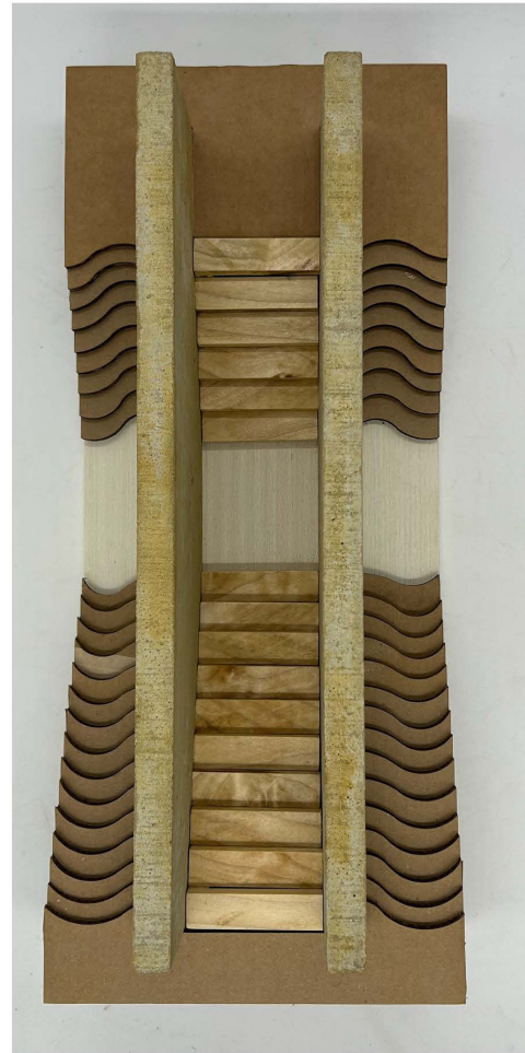
Test pieces for iron reaction with iron embedded in the mortar
