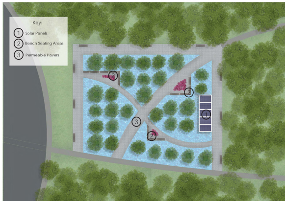
Enlarged plan of the well on the Swamp Rabbit Trail shows variety from the well that connects the parking garage, the use of solar panels, and placement of benches that allows for parking but a view of the water and trees.
