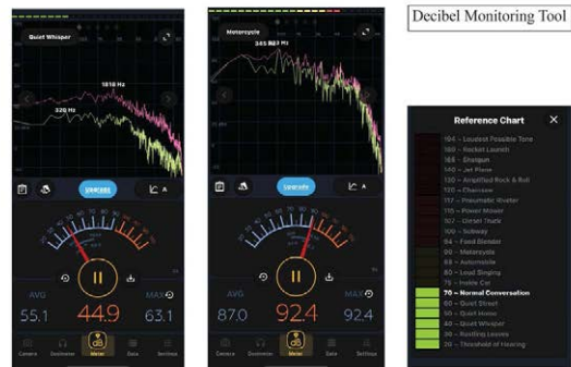
Figure 20: Screen shots of decibel meter application "Decibel X". The application allows the user to record audio data. The application can record sounds and calculate an average over a specified duration of time. The user can also take photos of the location while measuring sound. The app overlays location name, date and decimal readings on the screen This can be captured using the screenshot function of the smartphone. This app is free to download and many of the functions are free to use. Some premium applications require a subscription and 4.99 USD per month.
