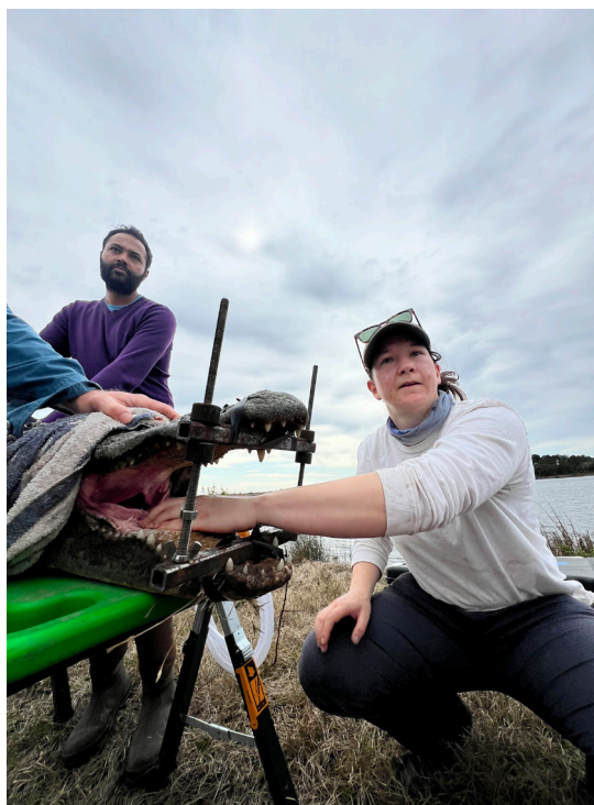
Miriam in the field with the U.S. Fish and Wildlife Service at the Cape Romain National Wildlife Refuge. The photo shows the deployment of a novel crocodilian jaw prop designed and used on this project. The design and testing of this device was published in the Wildlife Society Bulletin June 2024.
