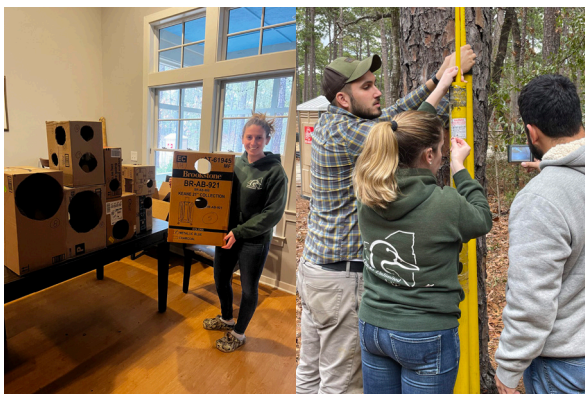
Figure 2. Two-person operation of a wireless cavity monitoring system capable of measuring external and internal dimensions of wood duck nesting cavities.
