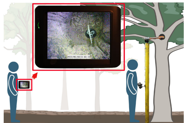
Figure 2. Two-person operation of a wireless cavity monitoring system capable of measuring external and internal dimensions of wood duck nesting cavities.
