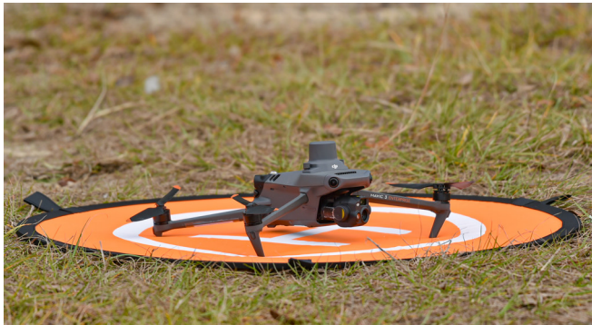
Figure 3: DJI Mavic 3T drone with RGB and thermal camera.
