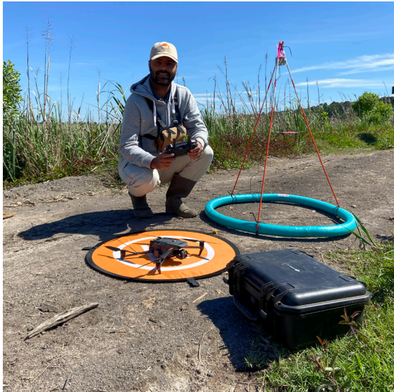
Image 1: Deploying and retrieving ARUs mounted on top of a designed multi-terrain lightweight floating platform in inaccessible areas using a drone.
