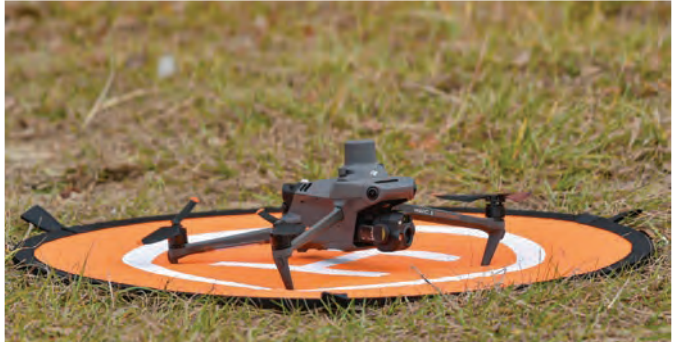
Figure 2: DJI Mavic 3T Enterprise drone deployed for aerial waterbird surveys in South Carolina’s coastal wetlands. Equipped with high-resolution and thermal imaging.
