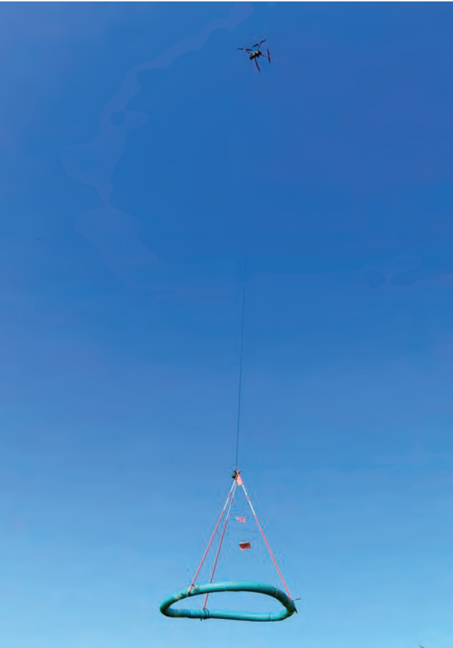
Figure 5: Using a drone to deploy and retrieve the floating ARU platform in otherwise inaccessible wetland areas.
