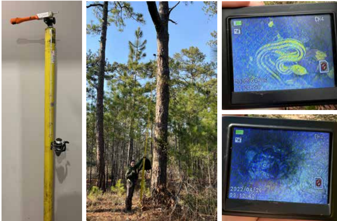
Figure 1. Wireless Cavity Inspection Camera (David Luneau, www.ibwo.org , Little Rock, AR, USA) fixed to a 15.24-m telescopic pole and modified to collect internal cavity dimensions and monitor cavity use.
