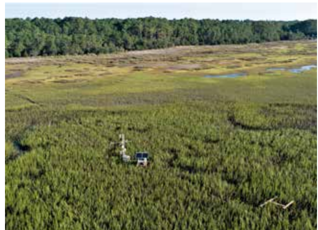
Figure 4. An eddy covariance flux tower in the North Inlet, open tidal salt marsh.
