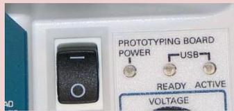
Turns the power to the *NI ELVIS* board on and off. The power LED lights up when the switch is turned ON.
