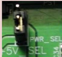
This allows to set the power input to the board by USB or Power Supply. We will set this jumper as shown in the adjacent figure to input 5V power to the board using the power supply.
