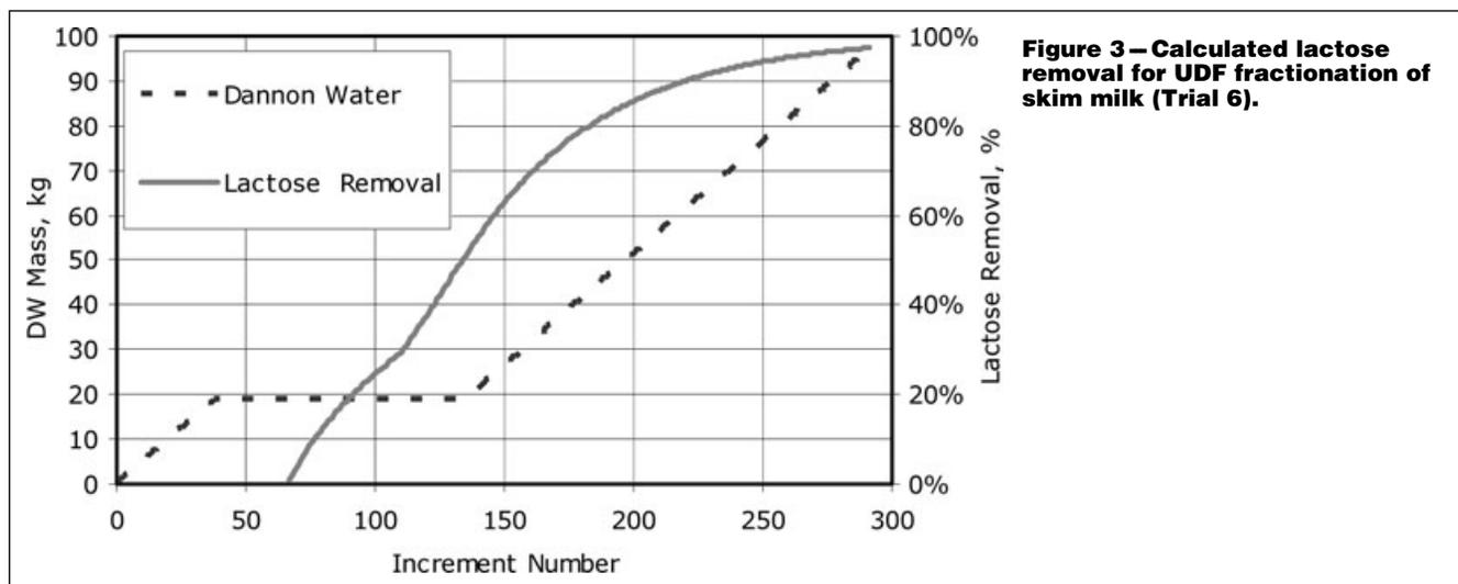
**Figure 3 – Calculated lactose removal for UDF fractionation of skim milk (Trial 6).**
