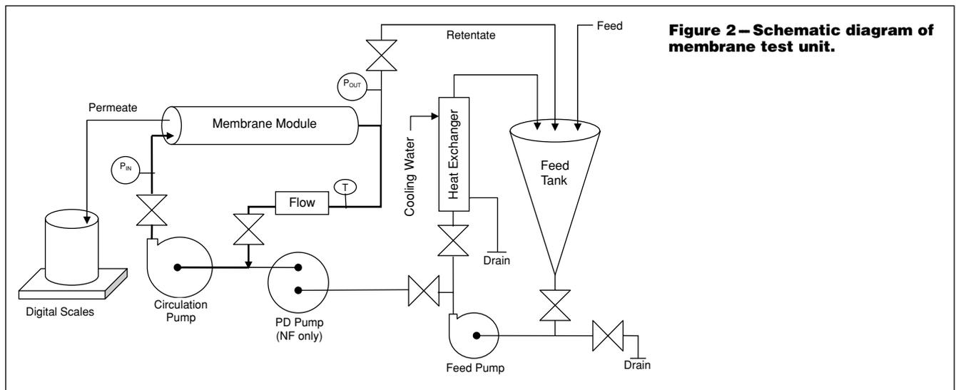
Membranes were cleaned in-place according to manufacturers' recommendations for cleaning and sanitizing agents, pH, temperature, and time. They were thoroughly cleaned and rinsed in-place with tap water between every fractionation experiment. The pumping system of the pilot-scale membrane test unit was controlled to provide a circulation rate of 61 kg/s.
