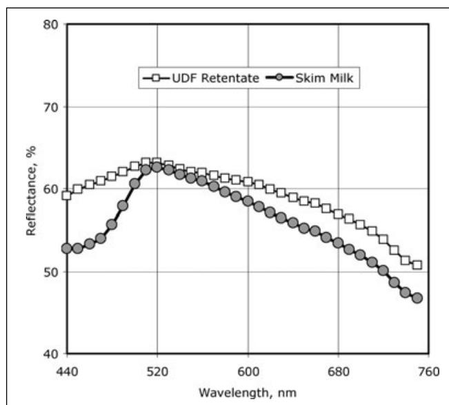
Figure 6 – Surface reflectance of skim milk & UDF retentate as a function of wavelength.
