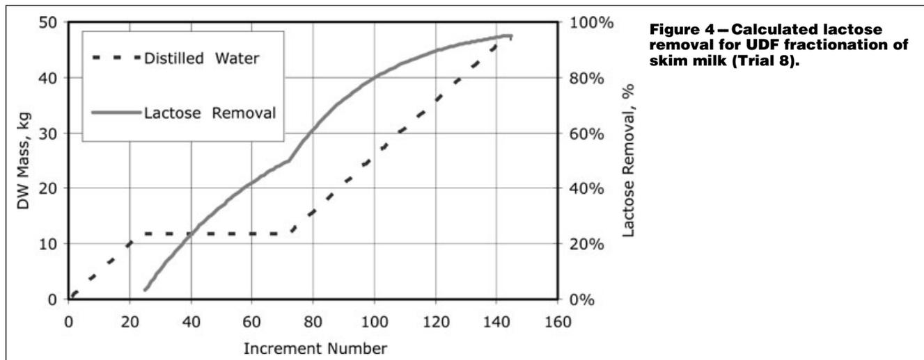
**Figure 4 – Calculated lactose removal for UDF fractionation of skim milk (Trial 8).**
