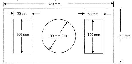
a) What punch force is required? (Note: both the external perimeter and the internal holes are punched from a larger sheet at the same time)
