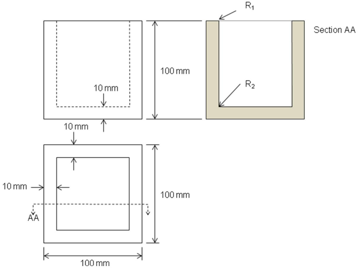
You will start with a block of 6061-T6 aluminum that is already milled to the dimensions of 100 mm X 100 mm X 100 mm and use a diamond coated high speed steel ball mill cutter with a 10 mm diameter. The bottom of the pocket should have a peak to valley surface finish ( $R_a$ ) of no more than 1  $\mu\text{m}$ . You should minimize the machining time for this operation. Please provide the following information for the pocket milling operation:
