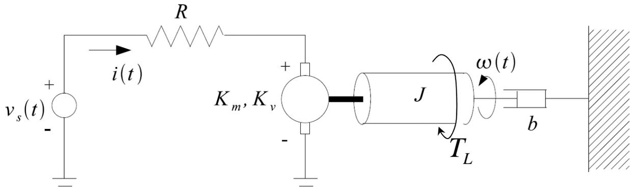
**Figure 3.** Servo control system for tracking antenna
