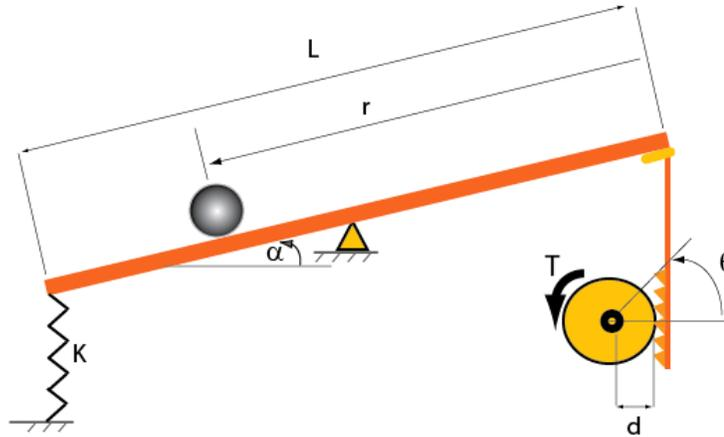
**Figure 1. Ball and Beam System.**
