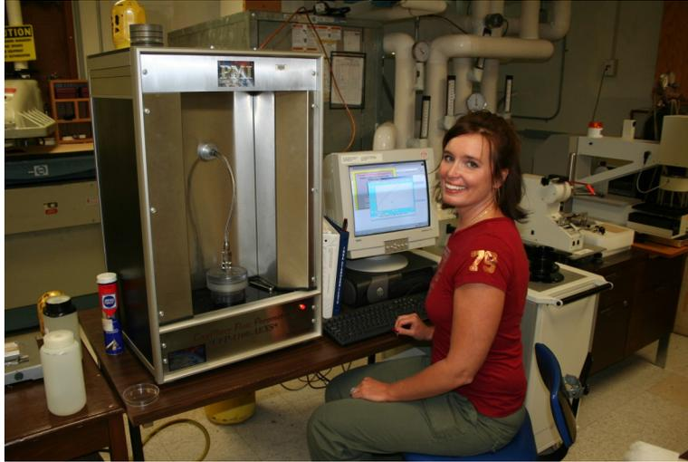
Capillary Flow Porometer
