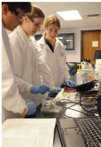
Dr. Delphine Dean and undergraduate students Matt Cupelli and Laura Wiles measure electrical conductance of alginate gels doped with nanoparticles.
