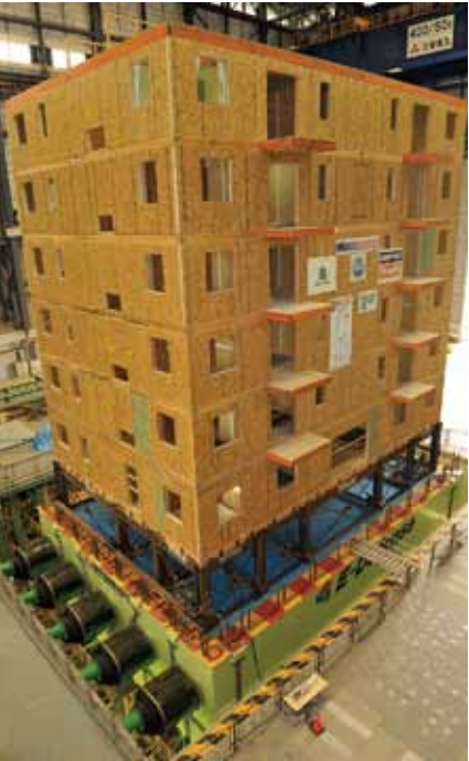
Wei Chiang Pang was among the team of researchers who convened in Japan's Miki City this summer to participate in the world's largest earthquake simulation ever performed on a light-frame wooden building. This earthquake experiment was part of the NSF NEESWood project.
