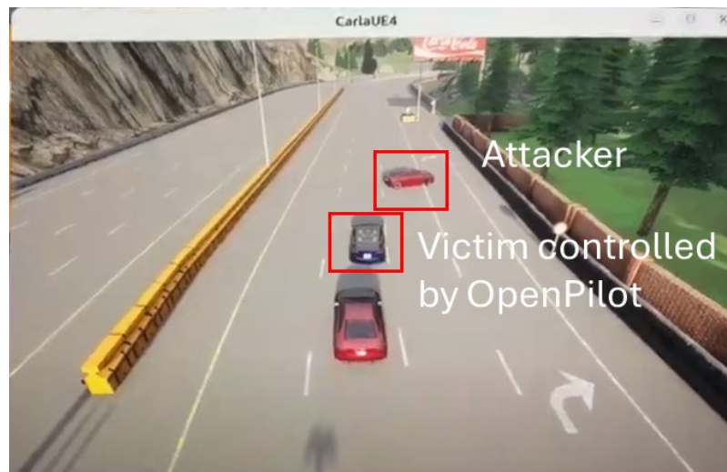
Figure 2: Illustration of the OpenPilot control software in the CARLA simulator
