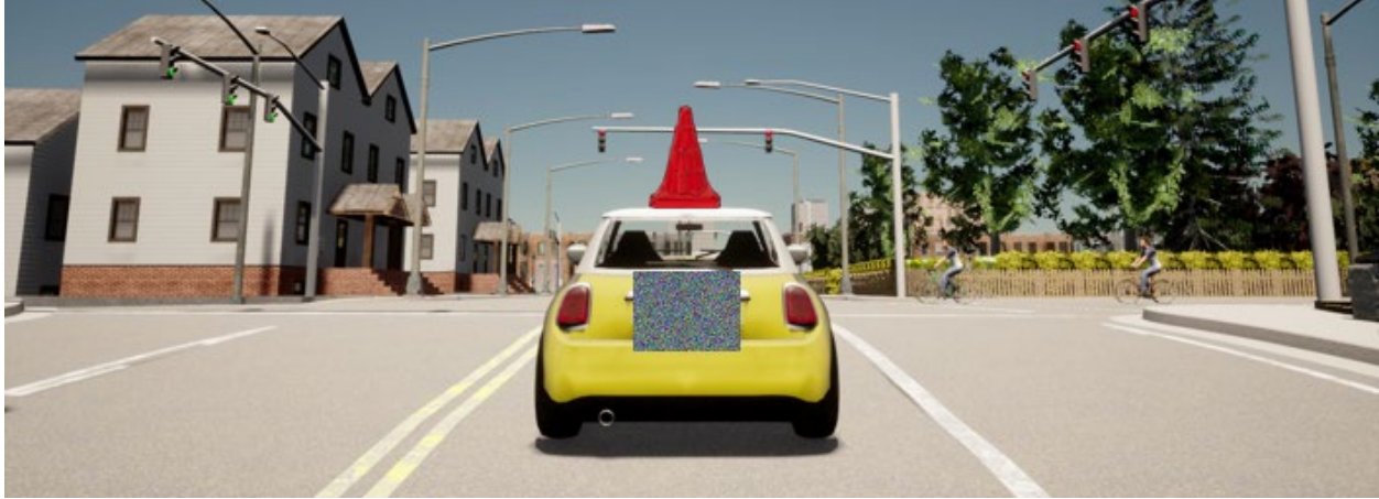
Figure 7: The front camera view w/ vision-lidar adversarial attack.
