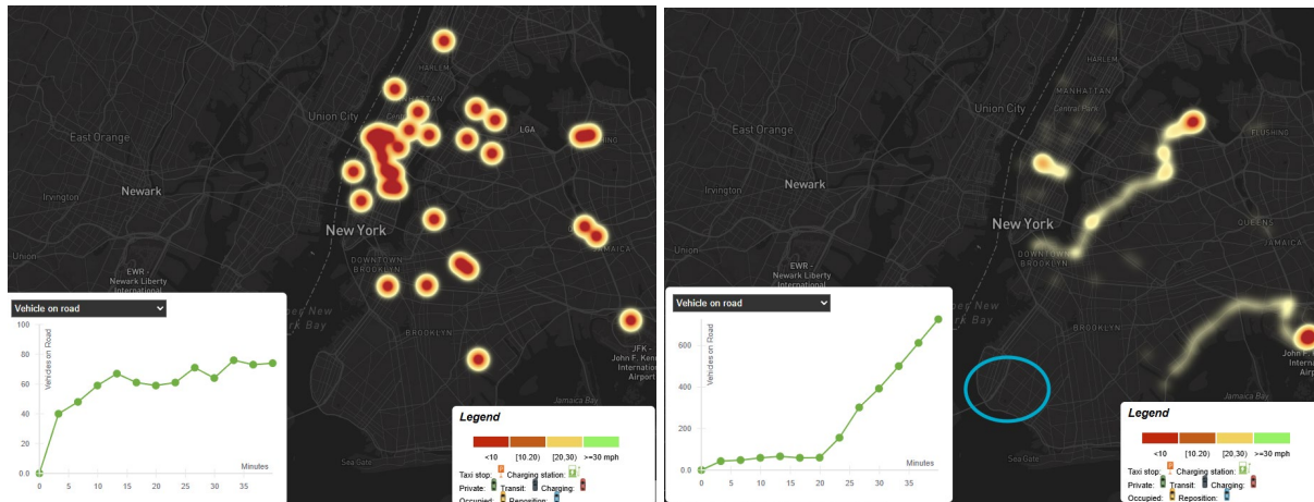
Figure 15: Repositioning vehicle distribution under normal (left) and attacked (right) cases. The blue circle marks the spoofed pickup zone
