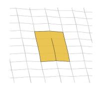
A single "cell" is comprised of 8 panels - all connected along the top and bottom seams, with one connected on the side.
