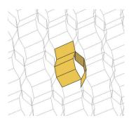
Then the side seams begin to fold every other, also causing a corrugated texture perpendicular to the first texture, which then forces the cell to open.
